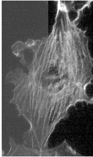
With the near-perfect sensitivity of Backside Illuminated Scientific CMOS sensors, the latest generation of scientific cameras have enabled imaging using only a few photons per pixel. Unfortunately, these minute signals are dominated by the natural Poisson variation in light levels preventing useful quantitation.
